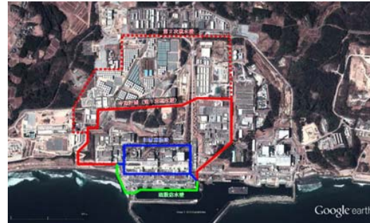
Fig. 7 Idea of multiple barriers to prevent leakage of radioactive water (proposed by JGS to IRID)
