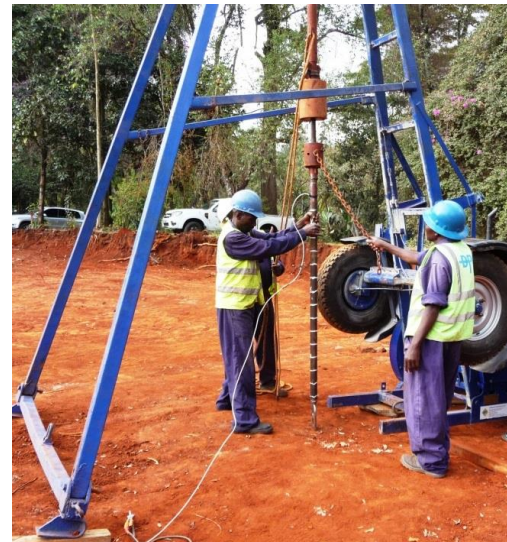
Fig. 7 DMT blade advanced by an SPT rig
