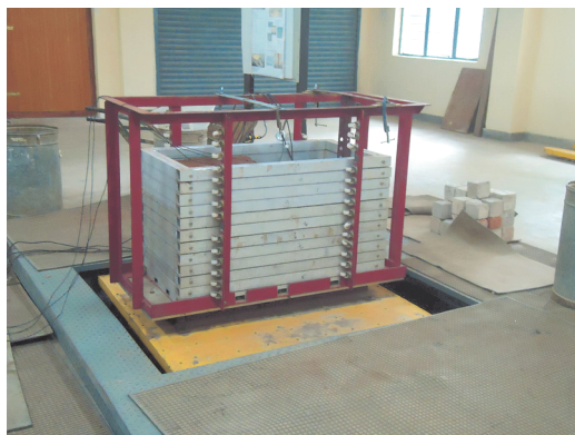
Figure 1. Laminar box mounted on shaking table
