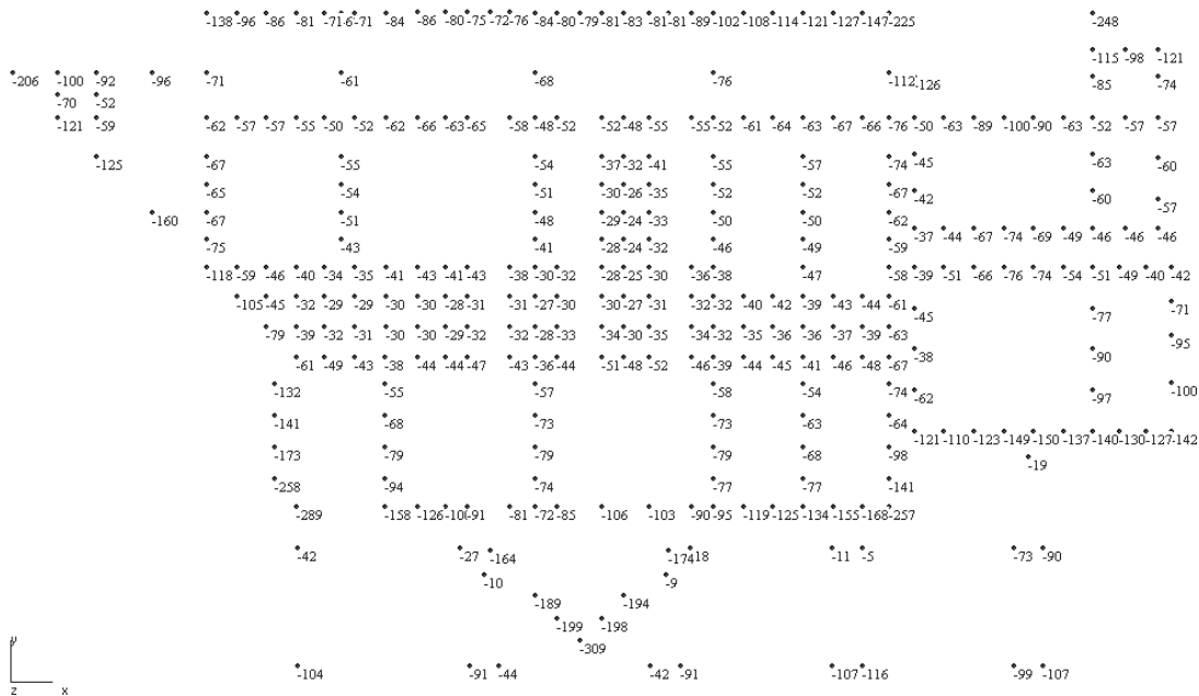
Fig. 28. Loads on piles (tonne/force) in the area of an adjoining 20-storeyed building.
