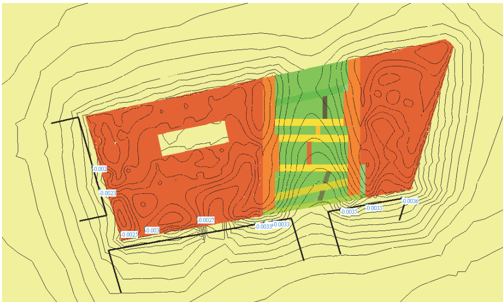
Figure 11. Settlements of adjacent buildings, m.
