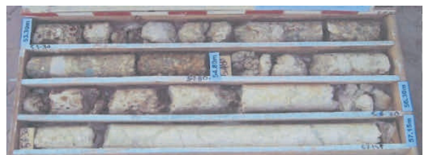
Figure 2. Triple tube (top) and double tube (bottom) core barrel drilling
