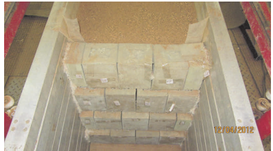
Figure 6. Typical modular block wall
