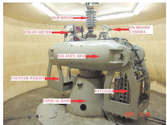
Figure 1. Photograph of NUS geotechnical centrifuge with the model package mounted on the platform
